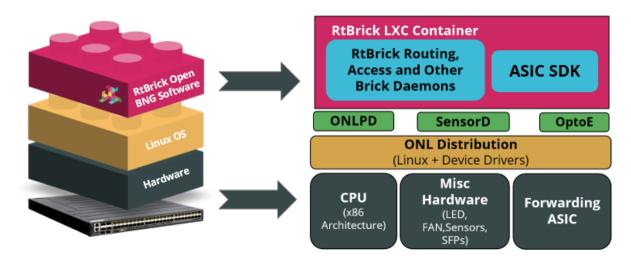
Platform hardware consists of forwarding ASICs and an Open Network Linux (ONL) operating system. A RBFS container that resides on top of this software includes all necessary packages to deliver access and routing protocols.
