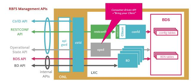
The illustration presents how the RBFS REST APIs communicate with various underlying software components. RBFS microservices, which perform various functions, are containerized in an open Linux container. RBFS APIs are generally categorized into Public Management APIs and Internal APIs. Public Management APIs include CtrID API, RESTCONF API, and Operational state API. These APIs are used by network administrators for managing and automating many of their network administration tasks.
