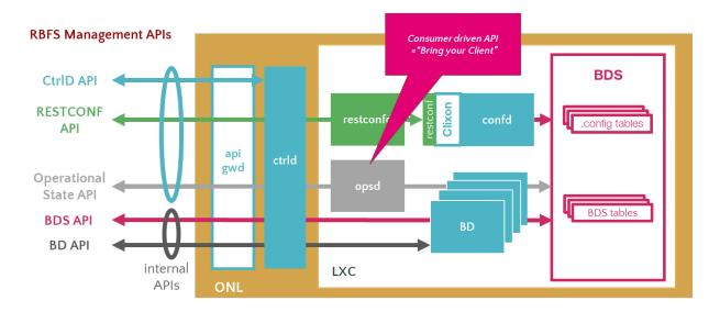
The illustration presents how the RBFS REST APIs communication happens with various underlying software components. RBFS microservices, which perform various functions, are containerized in an open Linux container. RBFS APIs are generally categorized into Public Management APIs and Internal APIs. Public Management APIs include CtrlD API, RESTCONF API, and Operational state API. These APIs are used for managing and automating many of the network administration tasks.
