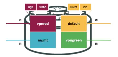
Each logical interface (ifl) is associated uniquely with a routing instance. If no routing instance is explicitly configured, the default routing instance is used. The interface association can be seen with the show interface address command.
