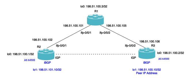
The BGP route for 198.51.100.10/32 will only be added to the routing table of router R2 if the IP address listed as the next-hop attribute is already reachable based on the information stored in the routing table. Additionally, the BGP route that is installed will contain a reference to the next-hop address 198.51.100.2 (refer to the figure above).
