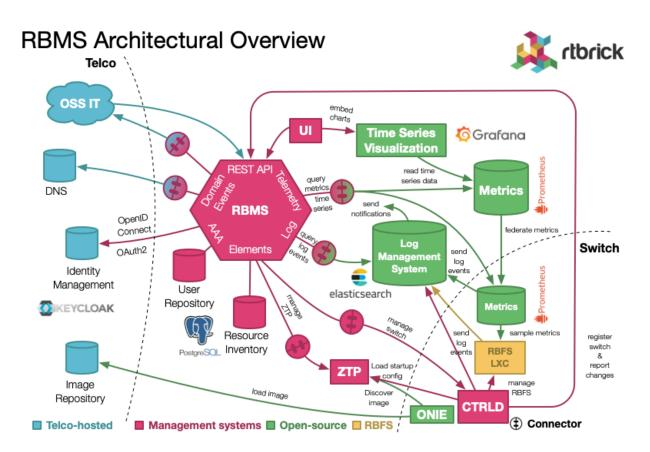
OSS-IT and RBMS UI manage the switches installed in the network. This includes to inspect the state of a switch but also to manage the switch configurations or to install a new software image.
