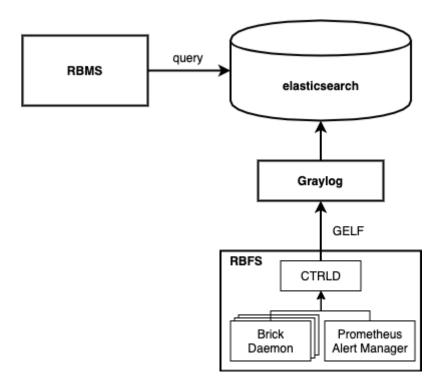
The CTRLD forms the egress node for all GELF messages. CTRLD receives log messages from brick daemons, augments the GELF message with the element name, element role, serial number and pod name and forwards it to the configured GELF endpoint. In addition, CTRLD receives all notification of the Prometheus Alert Manager running on the switch and translates them to GELF messages. Last but not least, CTRLD generates GELF messages to log events.
