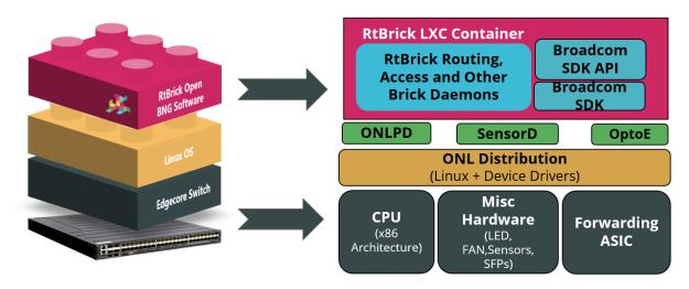
The platform consists of hardware based on forwarding ASIC and host operating system based on Open Network Linux (ONL). An RBFS container that resides on top of this software includes all necessary packages to deliver access and routing protocols.
