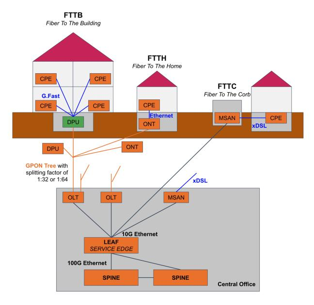
The LEAF and SPINE are bare metal switches running RBFS where the LEAF is responsible for service edge functionalities like PPPoE subscriber termination and the SPINE builds the actual fabric core. Multiple LEAF switches will be connected to a pair of spine switches.
