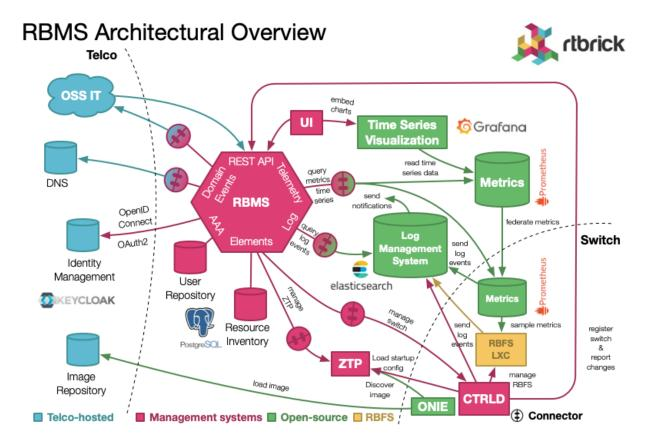
OSS-IT and RBMS UI manage the switches installed in the network. This includes to inspect the state of a switch but also to manage the switch configurations or to install a new software image.
